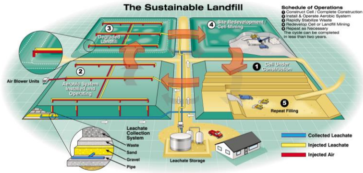
Figure 8: The Sustainable Landfill – Example Layout
